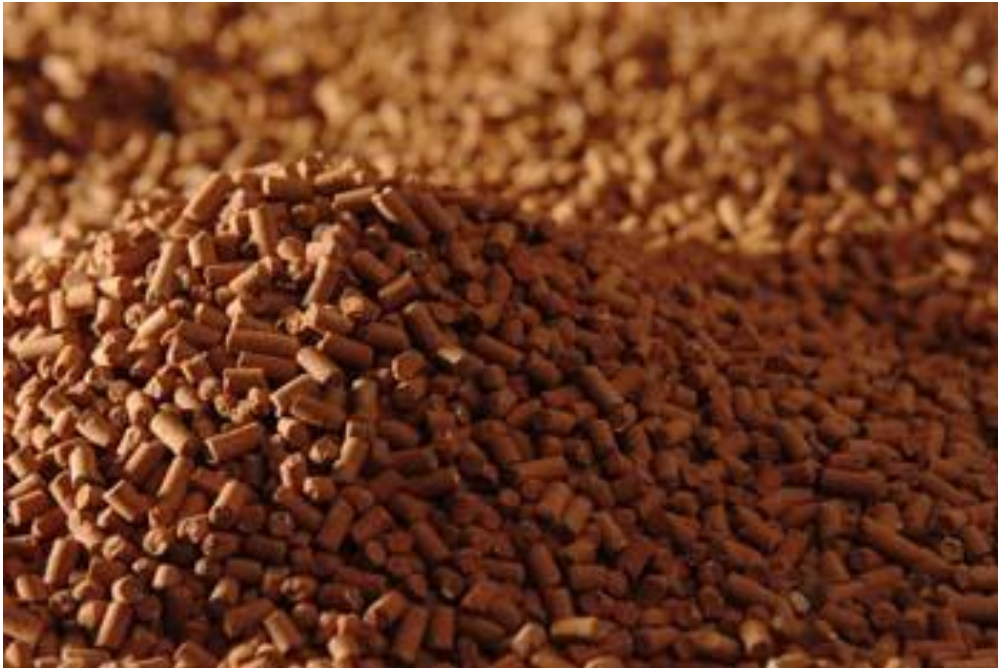
Catalyzer used in Isomerization Reactors
