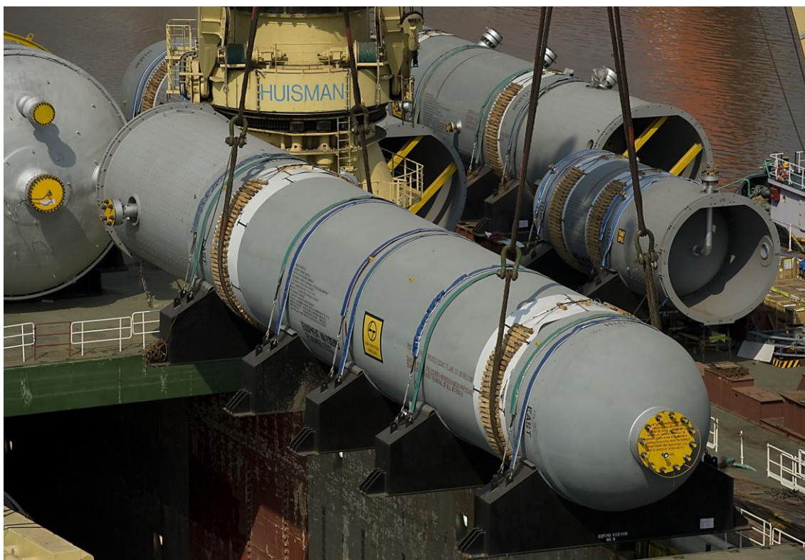
Sea transportation of Hydrocracking Reactors
