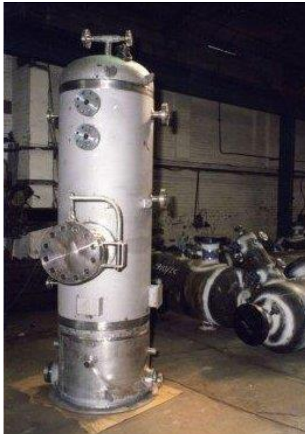
Example of a vertical vessel on a skirt
